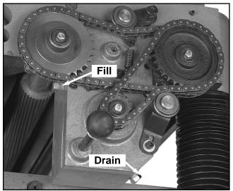
Figure 40. Gearbox fill and drain points.
